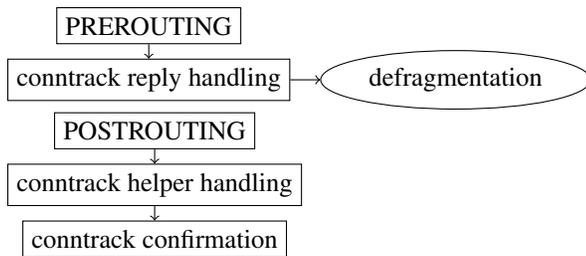
Figure 3: Hook placement for bridge connection tracking. Only Pre and Postrouting hooks are used. The conntrack reply hook also handles defragmentation.
