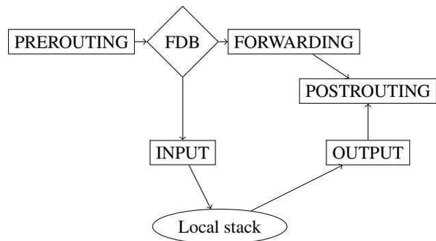
Figure 1: Bridge netfilter Hooks. Packets delivered to the local stack will be processed by the next protocol handler, e.g. the IP stack.
