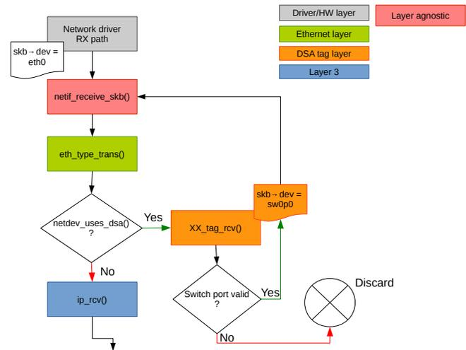
Figure 11: Processing the Switch Tag
