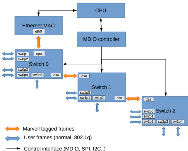
Figure 3: The D in DSA setup
