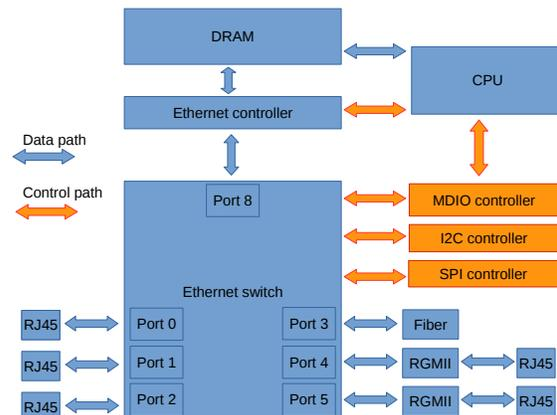
Figure 1: The Basic DSA setup
